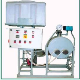
The Feed Funnel is filled with feed materials and it is operate when it starts feeding to the extruder barrel . At the same time the extruder motor is operated and the extruded product stabilises, the cutter motor is operated at proper speed to cut the extruded product to desired size. AFTER FINISHING THE OPERATION ABOUT 200 gm. Soyabean POWDER is passed without dies to clean the screw.
